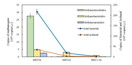
Fig. 4 Wash out of microorganisms with reducing HRTs.
