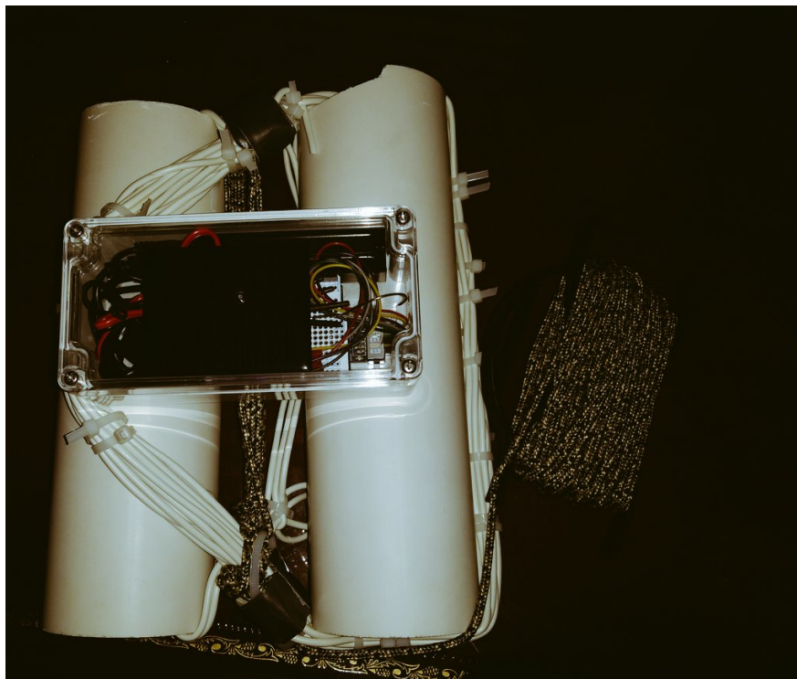
Figure 3: 2nd Version Test Deployment Data Logging Buoy
