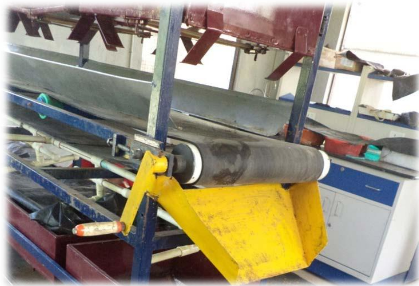
Figure 6: A typical module showing the arrangement at the base with which the content can be emptied. The guiding wheel is seen at the side.
