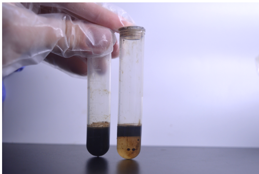
Figure S6. Optical images of crude oil-in-water emulsions formed by oil soluble PAA-PVK brushes (left) and water soluble PS-PAA brushes (right). Solid content for brushes content: 2 mg/mL.
