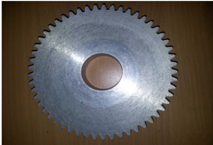
Figure 2 Machined Gear Blank and Al-Mg-Gr - SiC p Spur Gear
