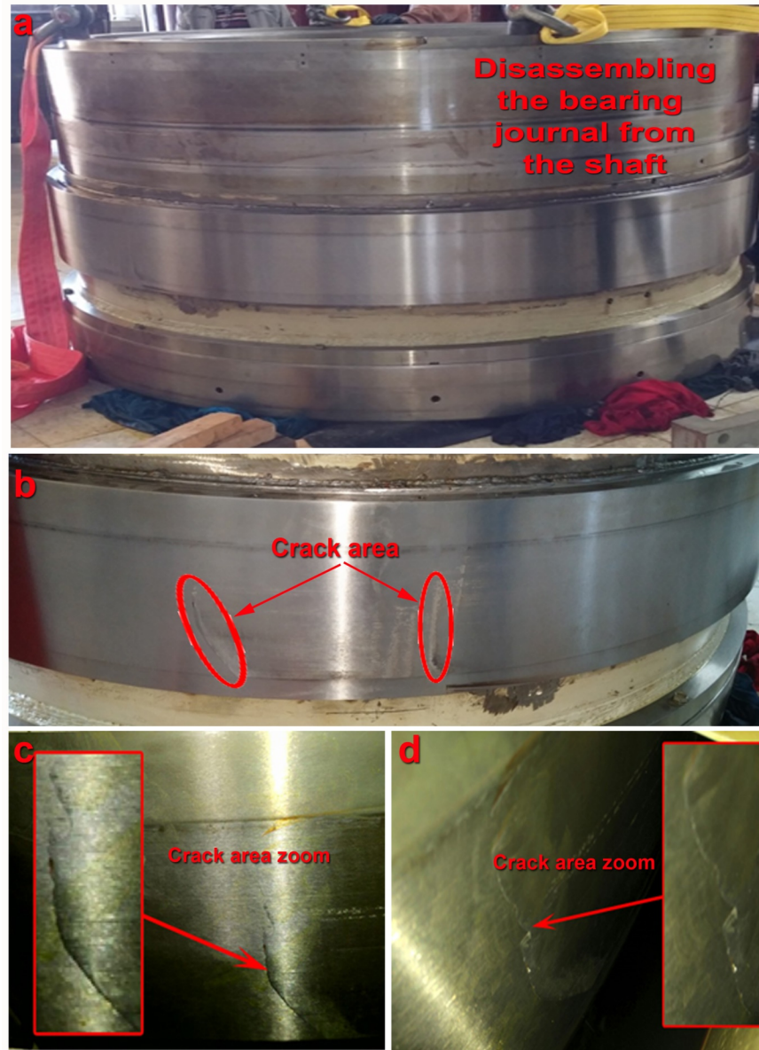
Figure 2. Image of crack areas on the bearing trunnion
