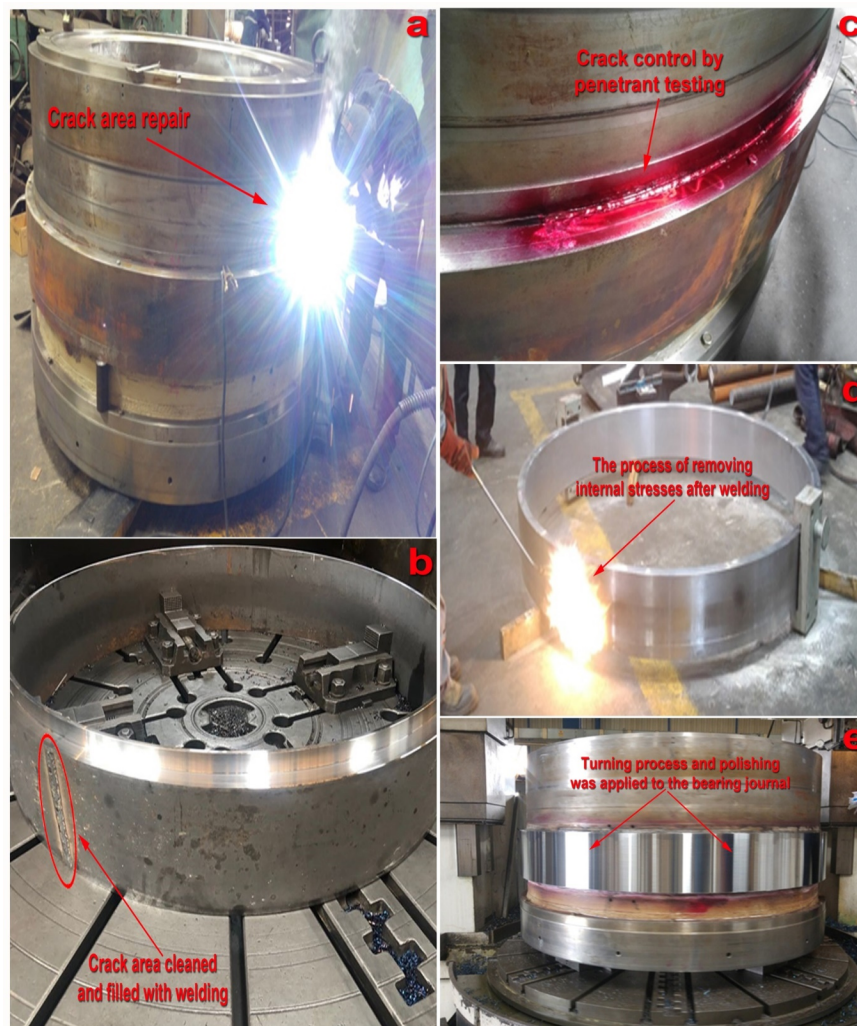
Figure 3.a) Repair of crack areas with oxyacetylene welding b) Cracks filled with weld c) Penetrant test for crack control d) Heat treatment on journal surface e) Turning and grinding process
