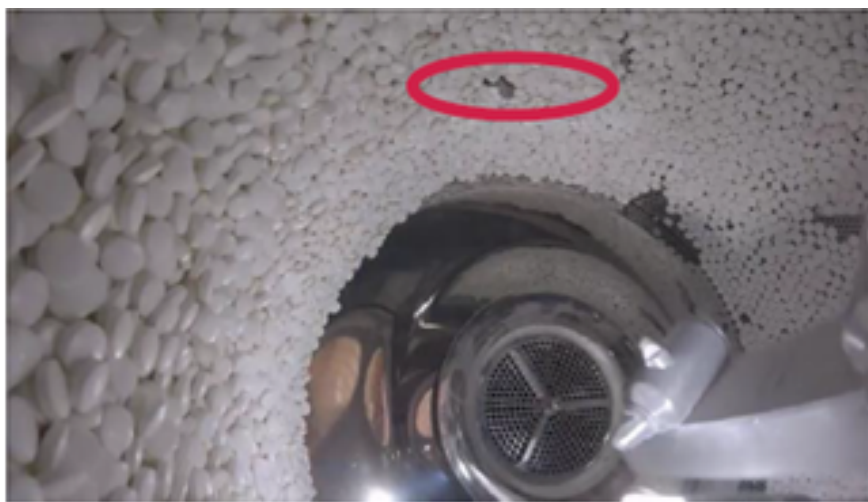
Figure 7: Maritime BioLogger inside the tablet bed in the ConSigma® 320 tablet coater.
