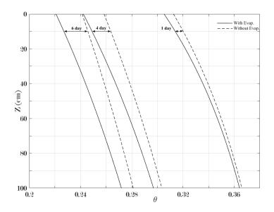
Figure 2. Comparison of soil water drainage with (solid lines) and without EV (dashed line).
