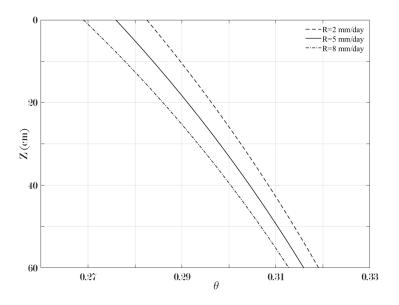
Figure 1. Example of drainage redistribution with deeply wetted homogeneous profile and EV solved analytically using different values of EV (2, 5 and 8 mm/day).
