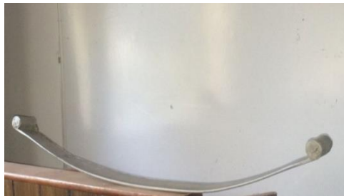
Fig.3.1: Composite Leaf Spring
