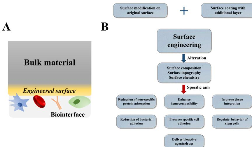
Figure 1. (A) Basic concept of surface engineering of biomaterials to control the interaction between living matter and biomaterials. (B) Surface engineering includes modification on original surface and additional layer coating to control over surface properties. By altering surface characteristics, various purposes can be fulfilled including enhanced biocompatibility, antibacterial ability, cells regulation and delivery of bioactive agents for specific applications.
