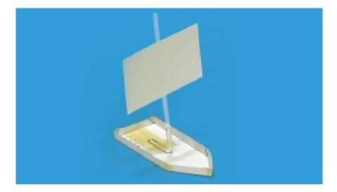
Students will design a boat body and study the effect of shape versus the load it can carry. This is looking at the force of buoyancy from the water compared to the load placed in the body of the boat. Next, they will look at sail design and see how to maximize the forward motion of the boat with different sail designs using a constant applied force to the sail.
