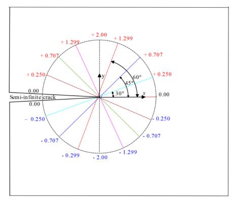
Fig. 5 Strain energy values around the semi-infinite crack (case of micro-crack is perpendicular to the semi-infinite crack); a)  $=\pi/2$ , b)  $= 3\pi/2$
