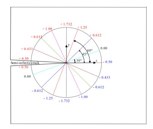
Fig.6 Strain energy values around the semi-infinite crack; a) = $\pi/3$ , b) =  $-\pi/3$
