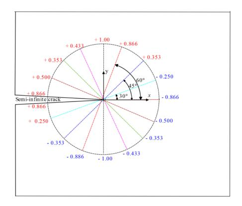
Fig.8 Strain energy values around the semi-infinite crack; a)  $=\pi/6$ , b)  $= -\pi/6$
