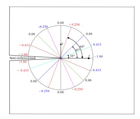
Fig.4 Strain energy values around the semi-infinite crack (case of micro-crack is parallel to the semi-infinite crack); a) = 0, b) =  $\pi$
