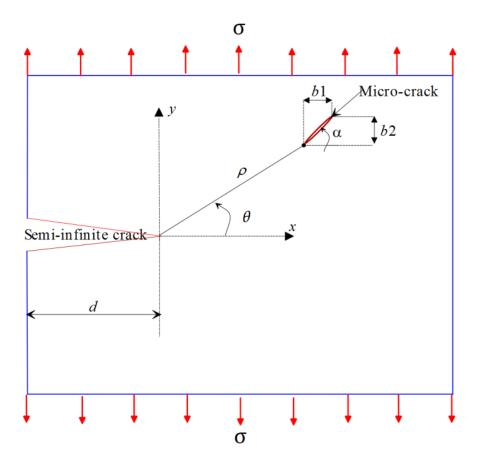
Fig. 1 Presence of semi-infinite crack and microcrack in the plane element
