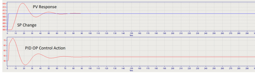
Figure 8 – CC and ZN control action with new PID tuning parameters upon a SP change
