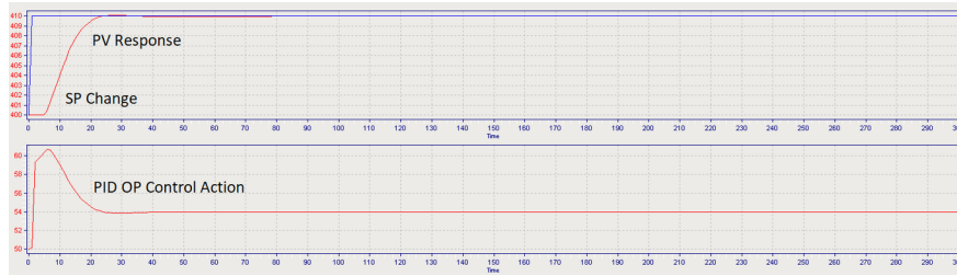
Figure 8 – CC and ZN control action with new PID tuning parameters upon a SP change
