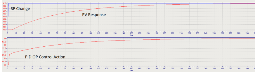
Figure 7 – Lambda and IMC control action with new PID tuning parameters upon a SP change
