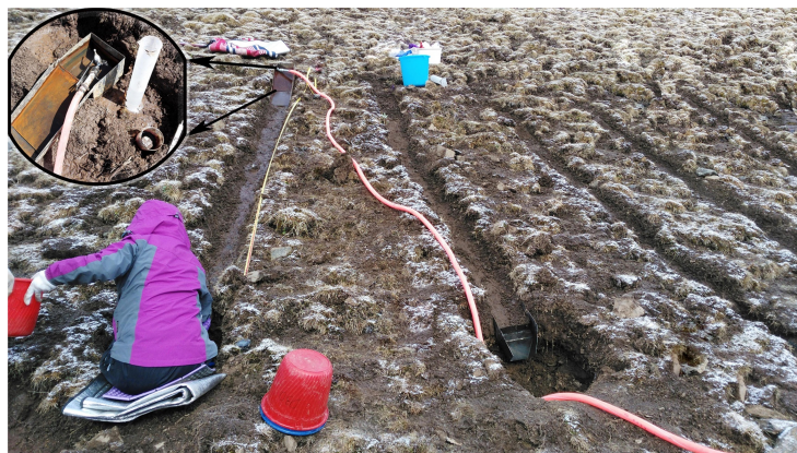
Fig. 3 Field experiments of concentrated flow erosion along a meadow hillslope.
