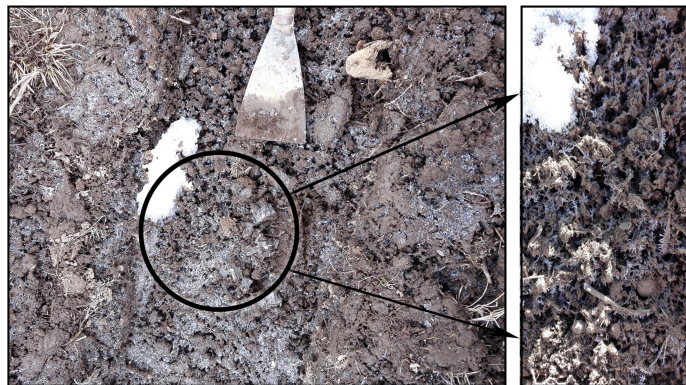
Fig. 9 The structure of the frozen soil surface with ice crystals in the soil voids.
