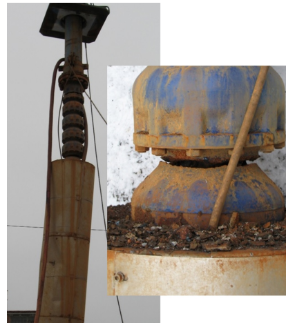
Figure 7: Damaged casing of a submersible drainage system pump used in a liquidated hard coal mine.
