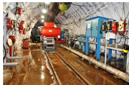
Figure 3: The view of water turbine and generator in pumping chamber [ Ing. Pavel Bartoš, FITE a.s.]
