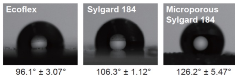
Figure S1. The hydrophobicity of materials was quantified using contact angle measurement. The contact angles of Ecoflex, Sylgard 184, and microporous Sylgard 184 were 96.1^\circ \pm 3.07^\circ , 106.3^\circ \pm 1.12^\circ , 126.2^\circ \pm 5.47^\circ respectively.
