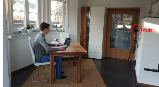
Fig. 10: Experimental setup for data recording with test person performing activity "working"
