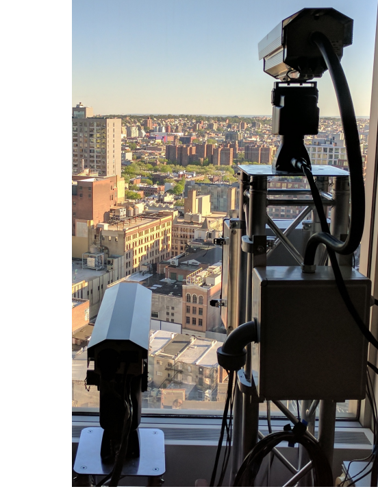
Figure 1. Figure 1. The hyperspectral camera (on the left) and the broadband camera (on the right) used to collect observed data. The cameras are shown here in the approximate orientation in which they captured data from a field of view south of the CUSP facilities at 1 Metro Tech Center, Brooklyn.
