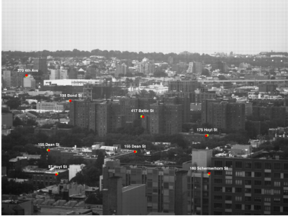
Figure 23. Figure 22. Eight fiducial points identified in the image (red dots) and projected LiDAR coordinates (yellow dots) used to optimize camera parameters
