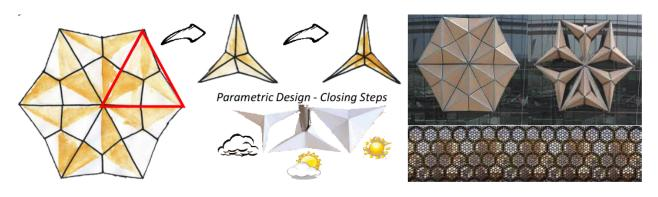
Figure 34: Mechanism of one module
