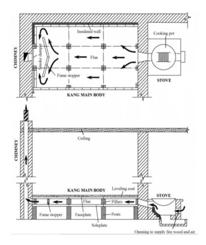
Figure 13: Keng Section and elevation (Sun, 2013)
