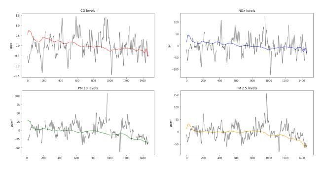
Figure 5: Change point detection curve fitted through data for a three month period
