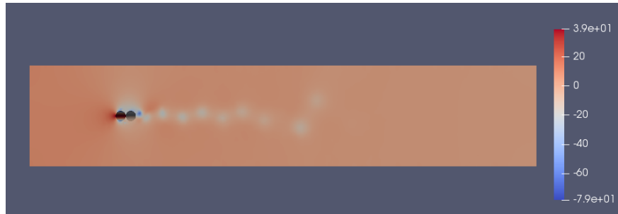
Figure 10: Pressure Profile for Cylinder Placement left and adjacent when A = 0.9
