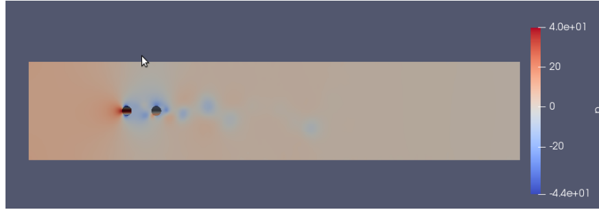
Figure 8: Pressure Profile for Cylinder Placement 0.2 meter to the right for A = 1.3
