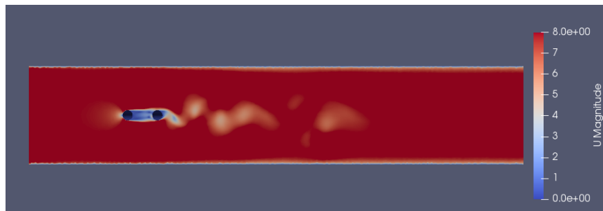
Figure 7: Velocity Profile for Cylinder Placement 0.2 meter to the right for A = 1.3
