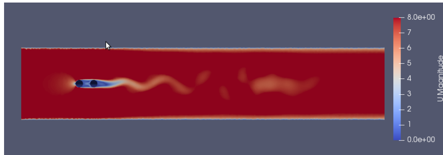
Figure 5: Velocity Profile for Cylinder Placement 0.1 meter to the left for A = 0.8
