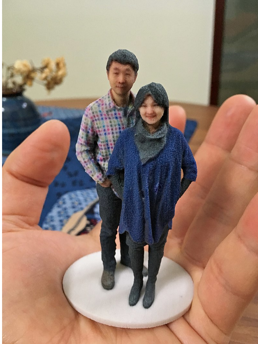
Figure 5: A 3D selfie in 1:20 scale printed by Shapeways using gypsum-based printing
